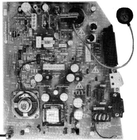
**Photo 2:** The Macintosh circuit boards. Photo 2a shows the analog board, while photo 2b shows the digital board. These two boards plus the video display, 3½-inch disk drive, and housing make up the main unit; only the keyboard and mouse are needed to make a complete Macintosh system.
