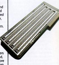
The SpeechLink will recognize a vocabulary of 64 words at one instant with an accuracy of from 85% to 100% depending on the words chosen, the user, the background noise, and the care with which the system is used. You choose which words you want recognized and program the unit — by speaking into it — to recognize these words for your voice. The words may be words or phrases up to 1.50 seconds long, a period of silence longer than 0.1 second indicates the end of the word.
